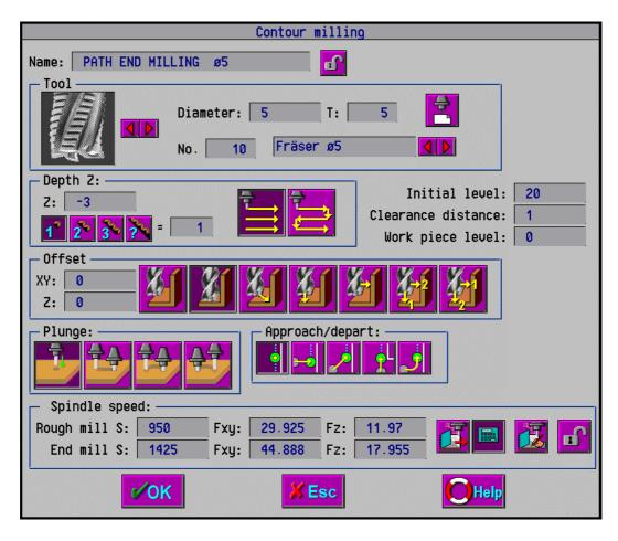
Notice that the cut depth is milled in 2 steps. This means that the mill passes through the path twice, for rough cutting all the material. During the simulation of the tool path, you will see that the mill drives more than once along the contour.
