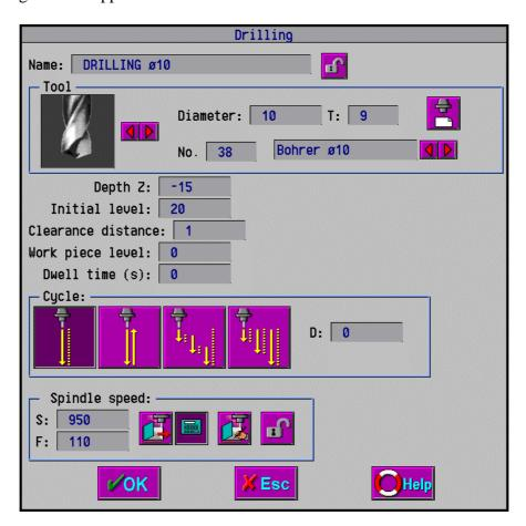
Fill in the window according to the above example. The correct drill is searched automatically according to the diameter of the circle. As Cycle you choose drill feed/rapid, which means that the tool cuts into the work piece in feed rate and then leaves in rapid traverse. Thereupon the holes are programed.
