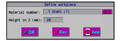
Determine the material of your workpiece here by scrolling back- and forward with the two arrows. All the materials defined in the material library will be enumerated. It is necessary for PrimCAM to know the specific material you are using for this piece to calculate the correct feed and speed rate automatically. Click the right arrow once, so the window will show 2 Al Mg Si0.5 (6) for instance, which stands for aluminium.
