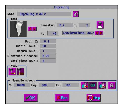
**Mode:** During the engraving, it often happens, that chips still remain in the path. With the option **double pass** the tool moves once more through the path in the opposite direction. The chips are removed, which results in a clearer engraving. But this option needs almost twice as much time and doubles the NC code size.
