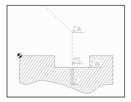
The **depth Z** indicates how far down from the workpiece level ZW the drilling should go. Z is normally negative and indicates the depth of a hole or a pocket.
