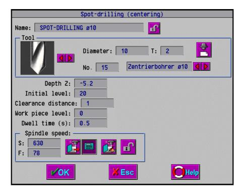
Fill in the window according to the above example. If you don't understand an entry in the window, move the mouse to it and press F1. A help window concerning the entry will be opened. Short explanations of the entries will follow:
